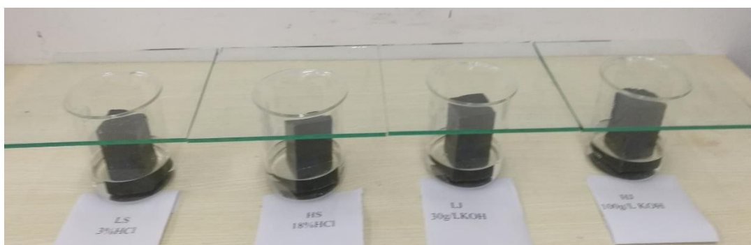
Figure 6. Chemical corrosion resistance determination
