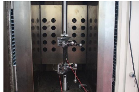
Figure 8. Tensile test at different temperatures
